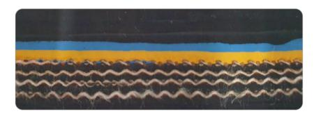
Bucket elevator conveyor belts have bolt holes to fix buckets along the entire belt length, making them apt to be torn easily and receiving pulled force with the buckets' weight. They also have a withdrawal force different from that of the ordinary belts in bending in connection with pulleys. Therefore, their carcasses mainly use polyester fabric that can address such problems. Steel cord is used when a highly powerful belt is required.
